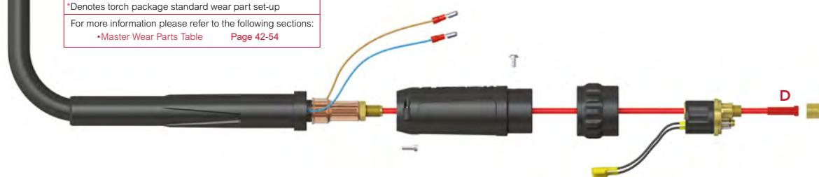
Rating: 350A CO<sub>2</sub> 320A mixed gas, EN60974-7 @ 35% duty cycle. 1.0 to 1.6mm wires
